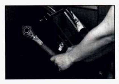
Remove the ratchet and extension by turning the wing nut counterclockwise. Remove the wing nut and retainer and take out the ratchet and extension.
